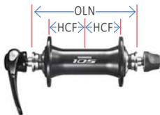
On a front rim-brake wheel, using a hub with equal-sized flanges, the HCF distance (and therefore the spoke length) will be identical on both sides of the wheel
