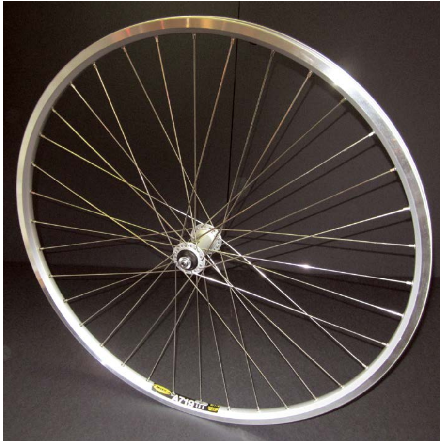
36-hole Mavic A719 wheel built onto a Shimano XT hub
