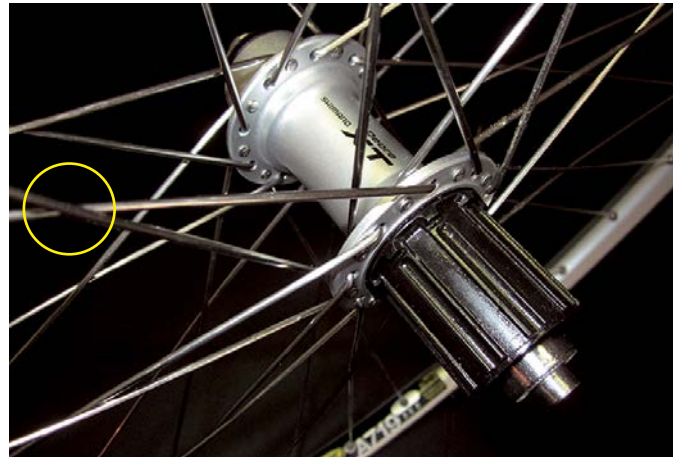
1 Symmetric lacing, cross-3 pattern
