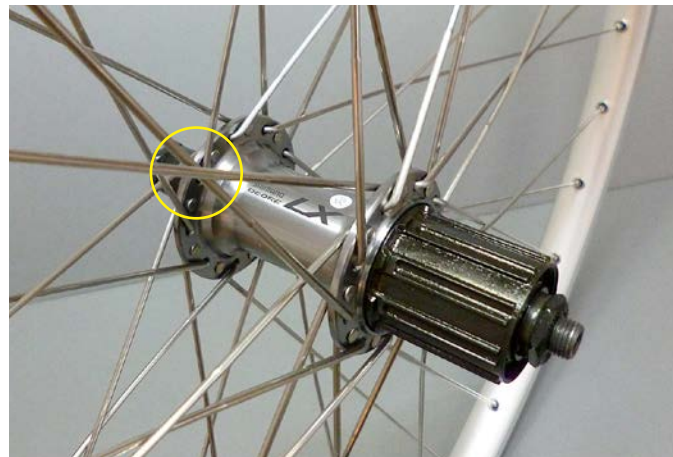
2 Asymmetric lacing, cross-3 pattern
