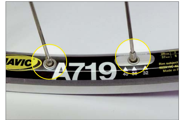
Spokes threaded onto nipples passed through holes in the rim
